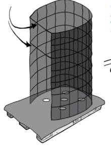
Cut wire re-mesh into dimensions. Add landscape fabric, cut to fit while still laying on the ground and fix it with wire.
