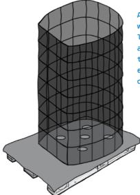
Add the door by attaching wires as hinges and firmly lock it into place with additional wires. (Leave them visible, so you can easily find them when opening the door).
